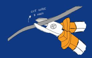
1st step: cut the 2mm wire in parts 10-20 cm each
