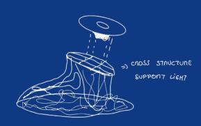
**4TH STEP:** CROSS **4** WIRES ON THE NECK, THIS WILL SUPPORT THE CD WITH THE LIGHT
